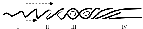
Figure 3. Schematic plot of formation of KHI billows and double-layer structure in a wind-sheared atmosphere. The dash-arrowed lines indicate horizontal wind. I, II, III, and IV point out the four stages of the distortion in the layer.
