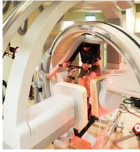
Fig. 1: The instrumented ergometer integrated with the dynamic fluoroscopy system for cycling exercise
