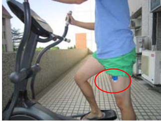
Fig. 5. Illustration of wearable wireless sEMG device worn on the lateral waist with electrodes placed on the left vastus lateralis.
