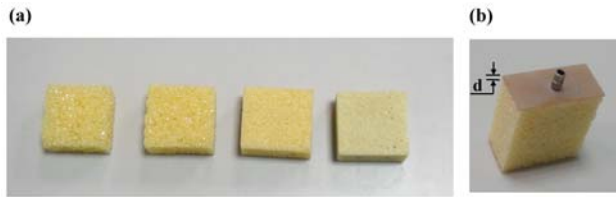
Fig. 1. (a) Artificial jawbone specimens of trabecular bone with elastic moduli of 12.4, 23, 47.5, and 137 MPa (from left to right). (b) Cortical shells with various thicknesses ( d=0, 1, 2, and 3 mm) were attached to trabecular bone with an elastic modulus of 23 MPa.
