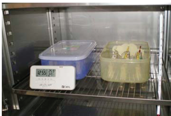
Fig. 3. Both groups were stored in a 27°C incubator; a thermometer (KOKA, KT-169, Taiwan) was used to monitor humidity.
