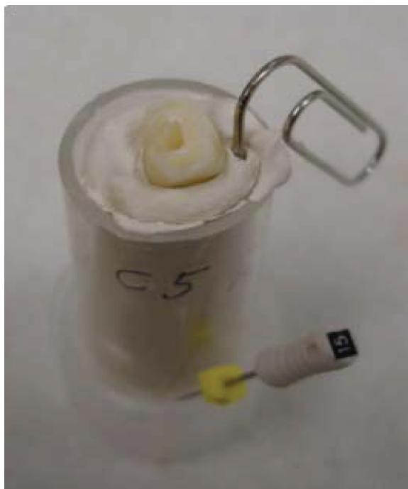
Fig. 2. A paper clip was inserted into the alginate to simulate an electric circuit in the oral cavity.
