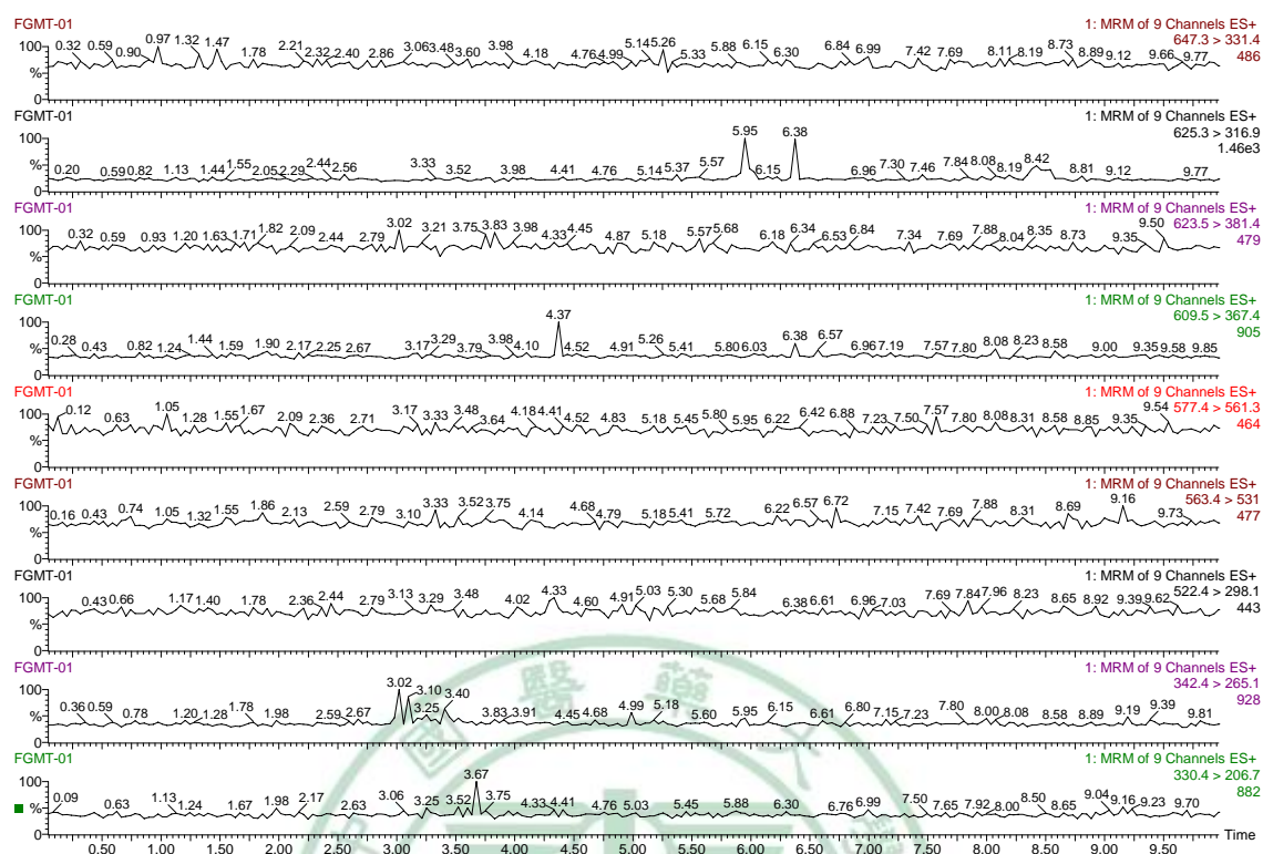
Fig.61 :The MRM chromatograms of Muh-Fangchi-Tang (木防己湯濃縮散) dry extracted preparation and the tested result of containing none of the 4 kinds of Fangchi herb (Formula label : Cocculus )
