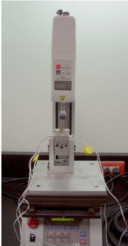
Fig. 3. (a) Application of forces to the top of the implant by a loading machine. (b) Two rosette strain gauges were attached to the bone surface buccolingually near the implant. 91x89mm (300 x 300 DPI)
