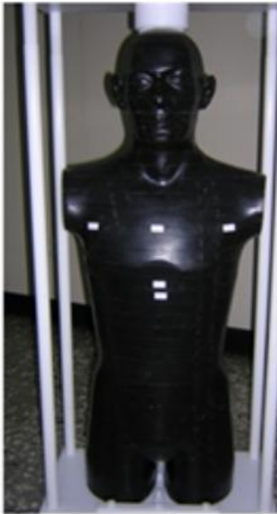
Figure 1. The photo of Rando phantom (left) and its CT image (middle). In the right is the distribution list of TLD measurement points inside the Rando phantom.
