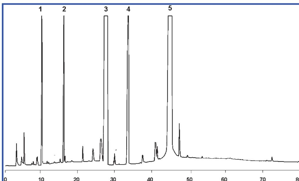
**Figure 1.** Analysis profile of garlic oil by gas chromatography. Diallyl sulfide (peak 1), methyl allyl disulfide (peak 2), diallyl disulfide (peak 3), methyl allyl trisulfide (peak 4), and diallyl trisulfide (peak 5) were quantified at 3.77, 2.75, 40.83, 7.17, and 38.93% in garlic oil, respectively.
