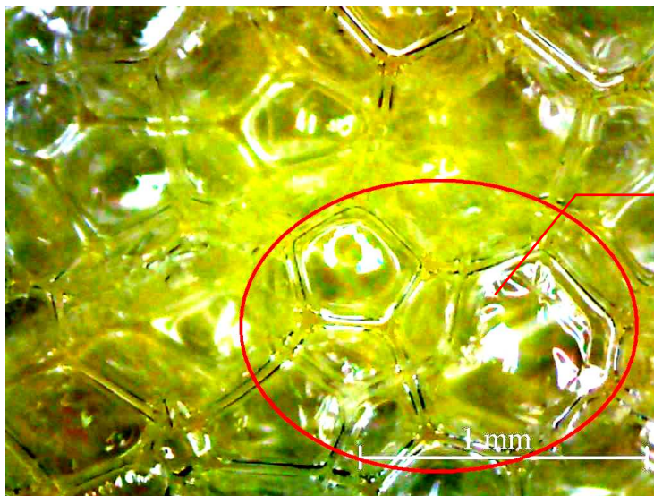
Figure 13 The illustration of the porous structure of the PU foam taken by optical microscope.
