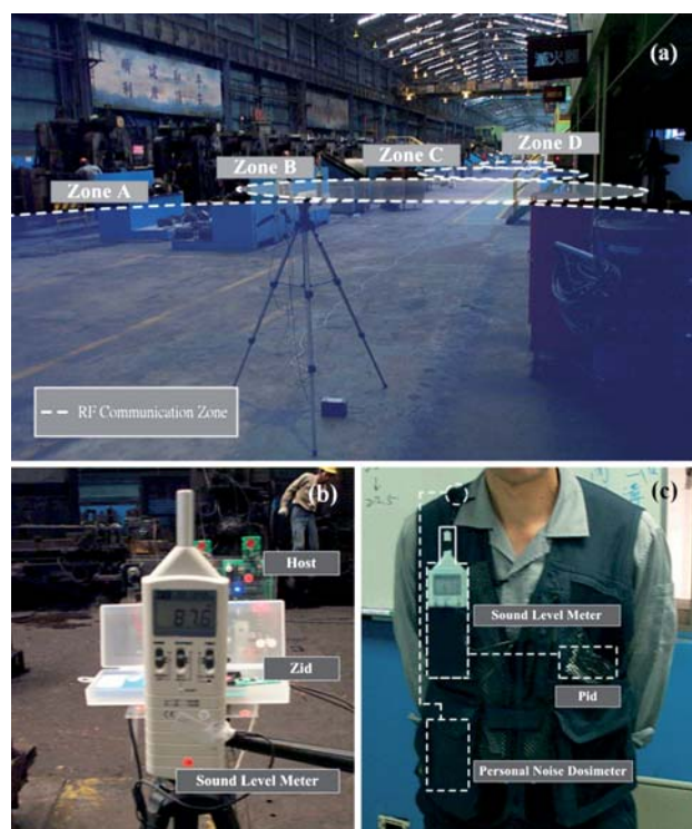
Fig. 3 Photographs showing the setup of field RFEMS: (a) the Host location and schematic diagram of the RF communication zones, (b) establishment of Host, Zid, and dosimeter in the microenvironment, (c) the worker vest with personal noise dosimeter, Pid and Sound level meter, dotted lines showing the location of each instrument inside the vest.
