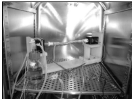
Figure 3. PGA Polymer Scaffold in the Bioreactor under Tensile Stimulation
