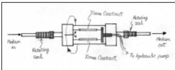
Figure 1. Draft Design for the custom-made bioreactor
