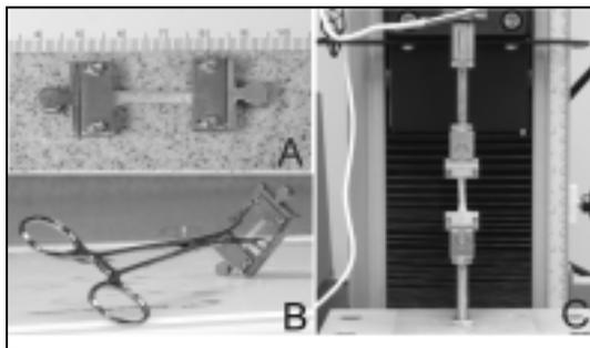
Biomechanical tests showed that with no tensile stimulation, the PGA scaffolds showed a tensile stiffness of about 90 N/mm. With continual tensile stimulation (+- 1% sinusoidal stimulation), the tensile stiffness in the PGA scaffolds increased significantly with time ( $p < 0.05$ ).
